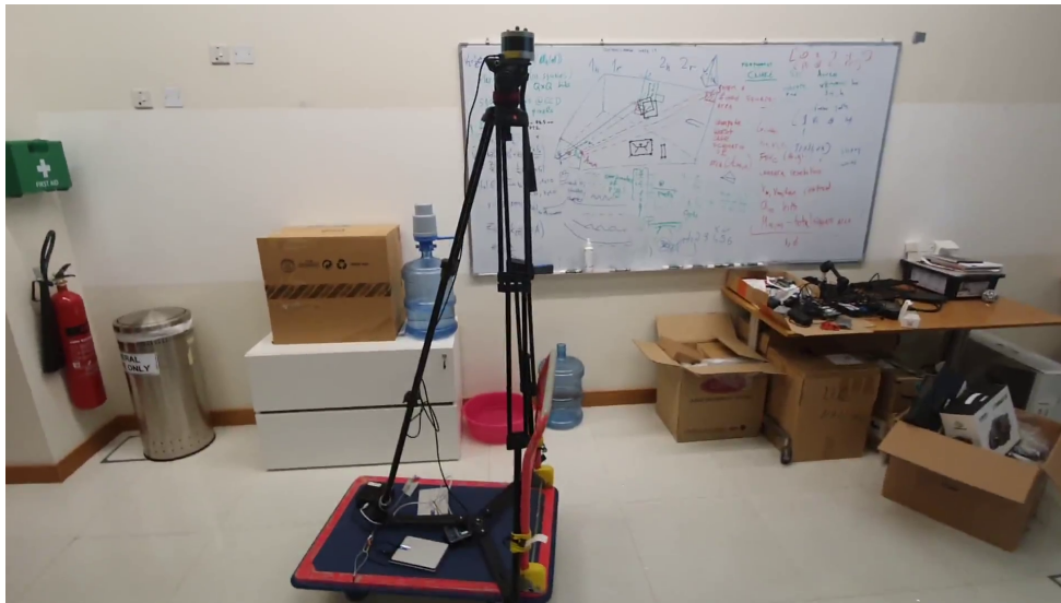
Figure 7.13: Trolley setup for 3D SLAM
