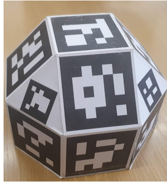
Figure 3.6: Aruco markers placed in a Rhombicuboctahedron solid
