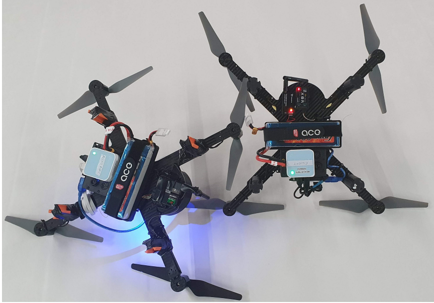
Figure 7.9: TP Link setup on drones
